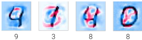
Figure 5. Targeted explanations Attributions generated explanation for a decision other than the one predicted. The class explained is indicated at the bottom of each sample – e.g, the first sample is a ‘4’ and the explanation is for the class ‘9’. As indicated in section 4.2, the red areas indicate that a black line should be added and the blue areas that it should be removed. More examples are available in the appendix.
